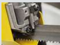
Precise guiding The saw blade is guided precisely using sanded carbide plates
