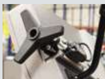
Saw blade break monitoring The saw blade tension is fitted with a saw blade tension and saw blade monitoring device
