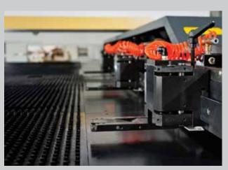
8 CLAMPING Movable pneumatic clamping.
